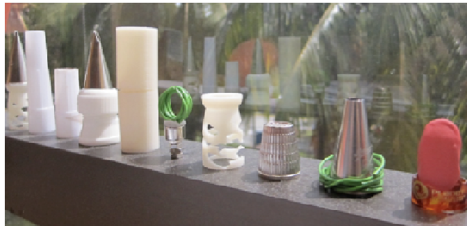
Fig.4. Design iterations for the wearable component. The final design is still being developed.
