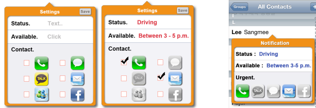
Fig. 3. Prototype of an interface that allows users to specify their availability and media preferences (left) and the manner in which it will be displayed to others (right)
