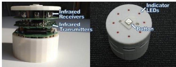
Fig. 2. Pebble Hardware. A pebble has 24 infrared transmitters, 8 receivers, 8 indicator LEDs, and a button. The infrared transmitters and receivers are arranged to cover all directions. The indicator LEDs are used to provide primitive feedback to the user. The button is used to receive user input.
