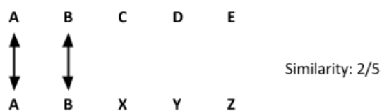
Figure 25. Similarity computing without a similarity measure (terms are either identical or infinitely different).
