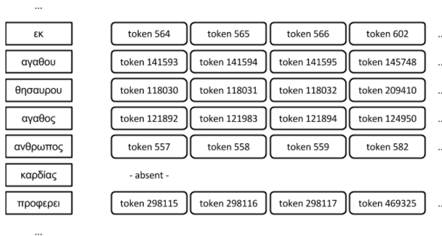
Figure 19. Representation of part of the generated index: each term is linked to all tokens (here, 3-grams) that contain it.
