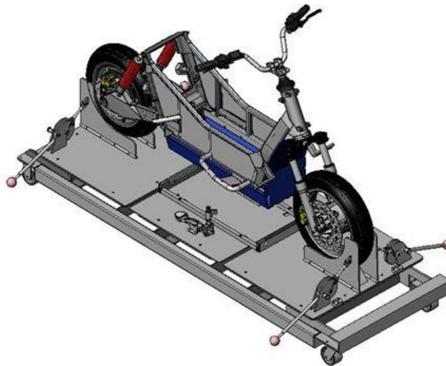
Fig. 2. Platform for assembling the scooter
