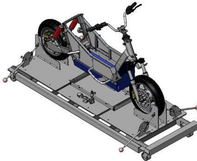
Fig. 2. Platform for assembling the scooter
