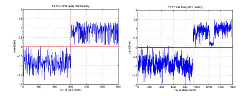
Fig. 1. Discriminant scores obtained via linear regression method with target values y=-1 for the faulty and y=+1 for the healthy state of the machine. Left panel: learning sample, first 300 faulty and next 300 healthy items. Right panel: testing sample, first 932 faulty and next 651 healthy items.
