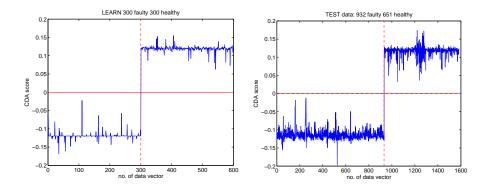
**Fig. 3.** Kernel discriminant function obtained from Gaussian kernel with  $\sigma=0.7$ . Negative and positive scores indicate the faulty and healthy state of the machine. Left panel: learning sample, first 300 faulty and next 300 healthy items. Right panel: testing sample, first 932 faulty and next 651 healthy items. Subsequent data items are linked by line segments. All items in both of the classes are classified perfectly.
