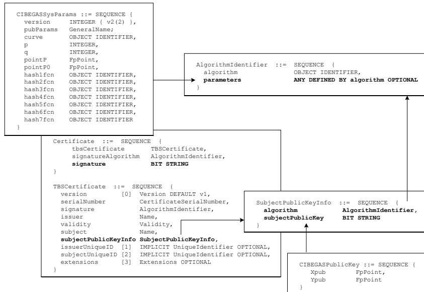
Fig. 4. X.509 certificate structure
