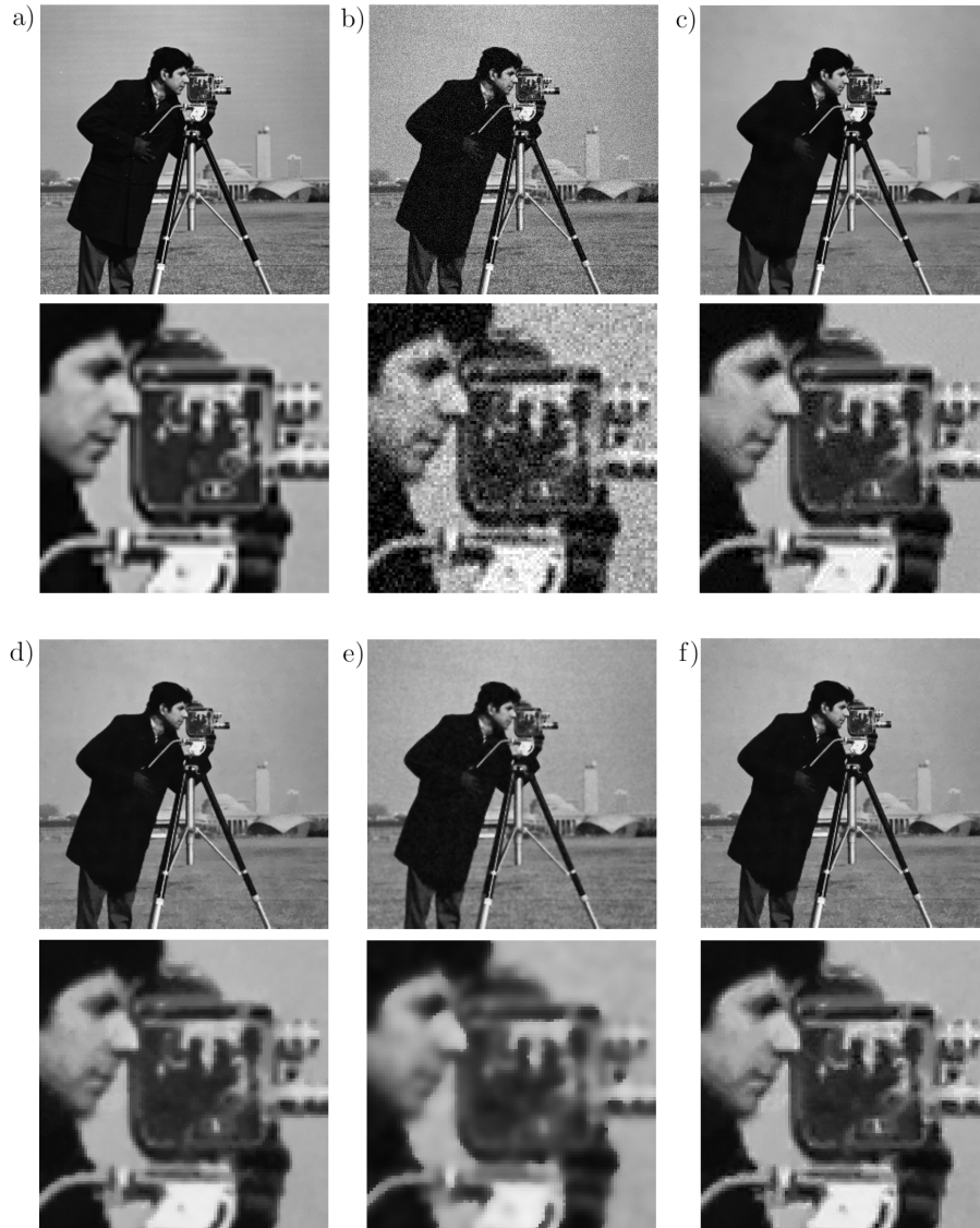
Fig. 4. a) Original image: 512 \times 512 (top) and 96 \times 96 (bottom) b) Noisy image: \rho = 20 c) NL-means: SSIM = 0.9214 d) Stochastic anisotropic diffusion: SSIM = 0.9144 e) Perona-Malik: SSIM = 0.8838 f) New method: SSIM = 0.9196
