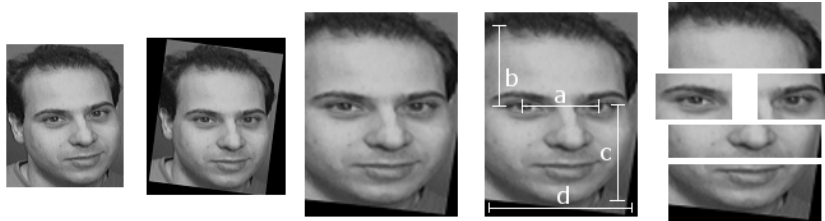
Fig. 2. Processing stages: original image, orientation normalization, scale standardization, salient point detection, facial areas extraction
