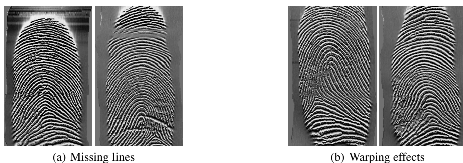
Fig. 3. Examples for distortions from actual acquisition problems.
