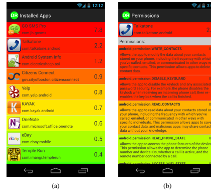
Fig. 13: DroidRisk Android App: (a) view of the list of installed apps with their corresponding risk levels, (b) view of the list of permissions requested by an app and their risk levels
