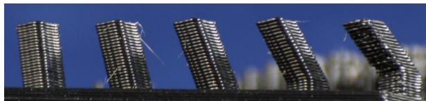
Fig. 16. - angles towards build-platform in FLM
