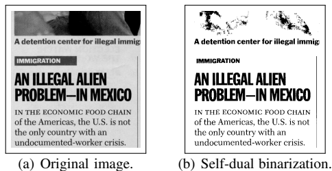
Fig. 9: Text segmentation with our method can be seen as a binarization technique, providing also reverse-video text.
