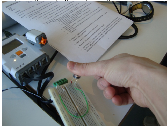
Fig.11. Testing and calibrating the light sensor
