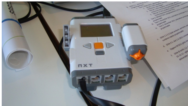
Fig.5. LegoMindstorms NXT as the platform for prototyping
