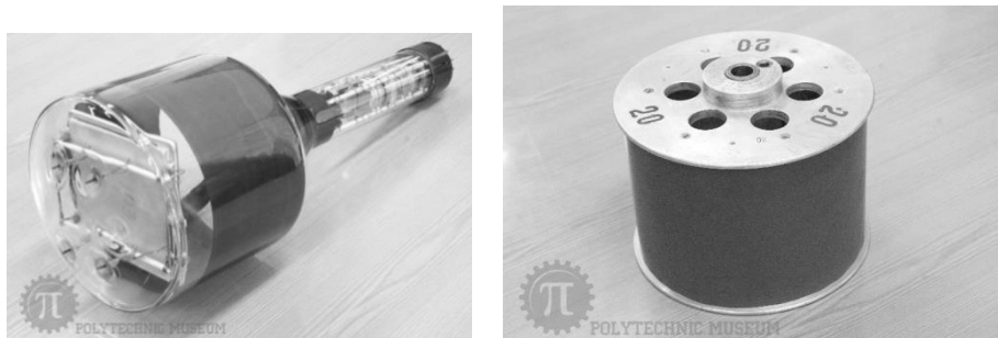
Fig. 4: The cathode-ray tube and the wide ferromagnetic tape the first Soviet serial computer “Strela”
