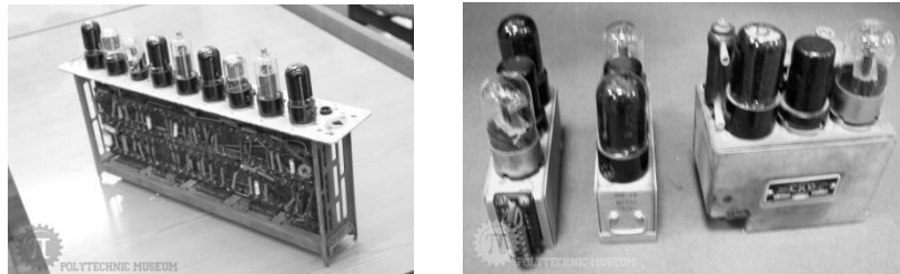
Fig. 3: Several processor blocks of the first Soviet serial computer “Strela”
