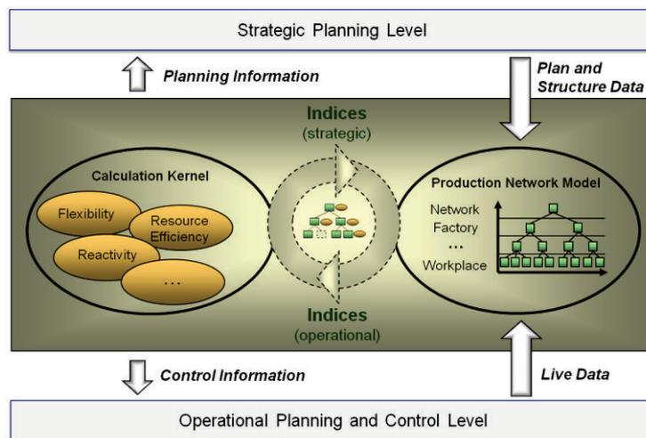
Fig. 1. Overview of the ecoFLEX approach (according to [2])
