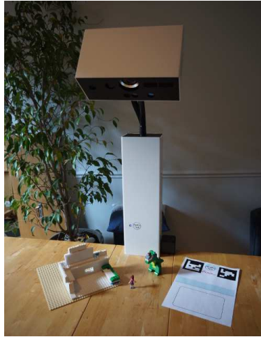
Figure 1. Photograph of the PapArt hardware by Inria Bordeaux: the prototype includes a projector, a RGB camera and a depth camera.
