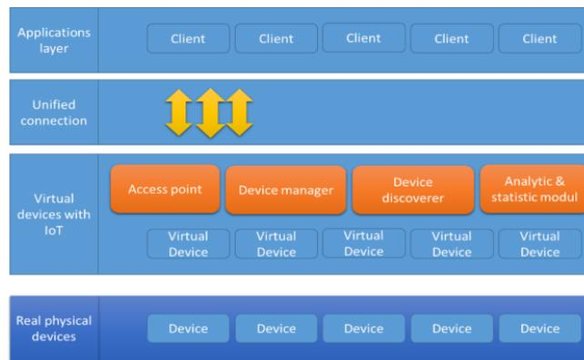
Fig. 3. Concept definition of IoT in the industry.
