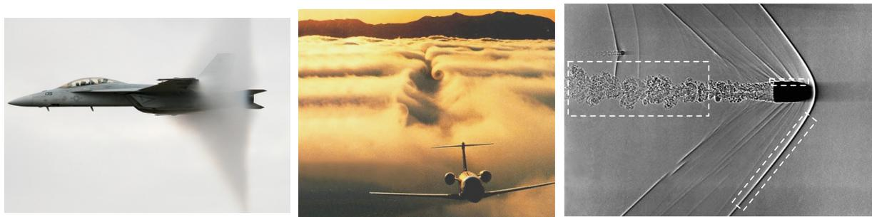
Figure 2: Left, shock waves (Mach cone) emitted by a supersonic F-14 fighter. Middle, turbulent wake of a transonic Falcon business jet. Right, schlieren picture showing the flow pattern around a bullet at supersonic speed. Dotted white squares exhibit different components of the flow features: boundary layer near body, shock waves in the far-field and turbulent flow in the wake.
