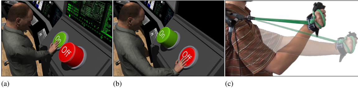
Figure 6. Pseudo-haptic effect simulating different levels of effort. (a) The button on the left is associated to an interaction coefficient k_i = 1 so the motion of the user's hand is unaltered when pushing it. (b) The button on the right is associated to a lower interaction coefficient k_j < k_i so the motion of the user's hand is slowed down. (c) User's posture when pushing on the first button. For pushing the stiffer button, the user compensates the speed difference by extending the arm furthermore (faded arm), which generates stronger haptic cues.
