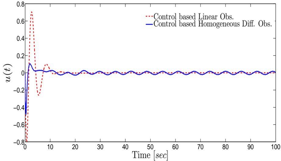
Figure 4. Control Signal. *The signal control based on the Luenberger observer spends more energy during the transient than the homogeneous differentiator observer. After this transient, the corresponding control signals are practically the same for both control approaches.*
