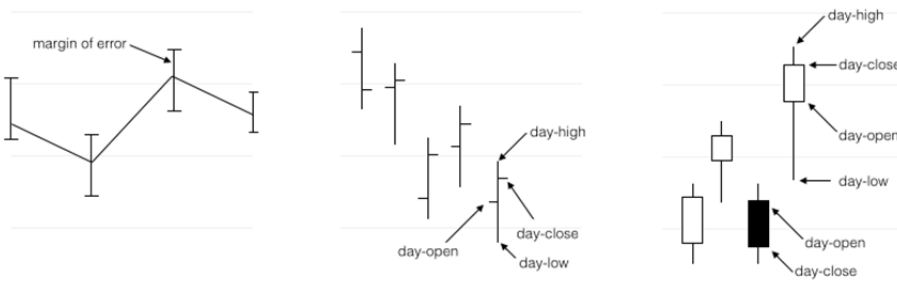
Figure 5 - Different techniques to incorporate range information, from left to right: error bars, envelopes and candlesticks. The examples are typical for use in financial market analysis.
