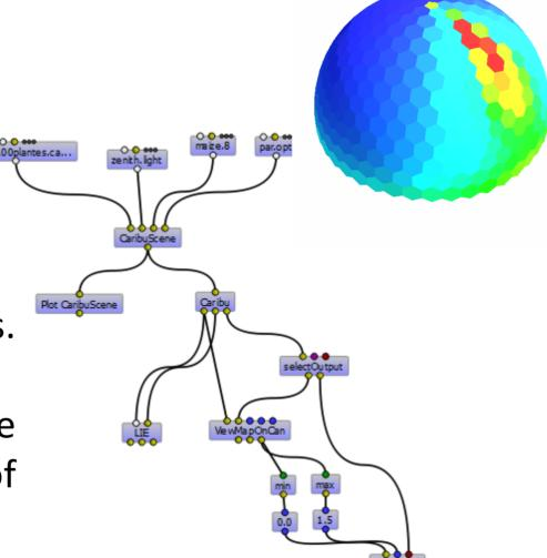
Using RT models requires an advanced expertise for a correct parameterization. The definition of standardized interfaces allow to ease this task by providing shared parameterization tools. We concentrate our effort on light sources by allowing parameterization of natural light condition from meteorological data. This tool implements the weather sky model of Perez et al. and offers a flexible 3D discretization of the sky.
