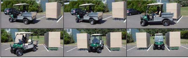
Fig. 14: Evolution of the sensor based perpendicular parking maneuver
