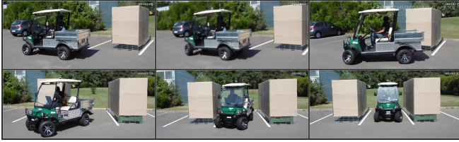
Fig. 14: Evolution of the sensor based perpendicular parking maneuver
