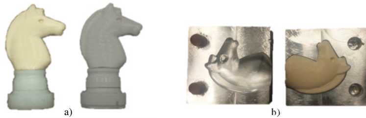
Figure 7. Knight quality issues a) Colour difference b) Fixture for hole drilling.
