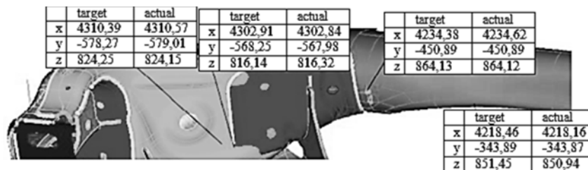
Fig. 6. Results of 3D measurement machine
