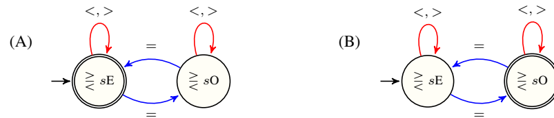
Figure 4.1051: Automata without registers for the (A) NB_STEADY_IS_EVEN and the (B) NB_STEADY_IS_ODD constraints; they respectively achieve an even/odd number of occurrences of the STEADY pattern on a sequence of n variables; transitions in blue correspond to a new occurrence of the STEADY pattern.
