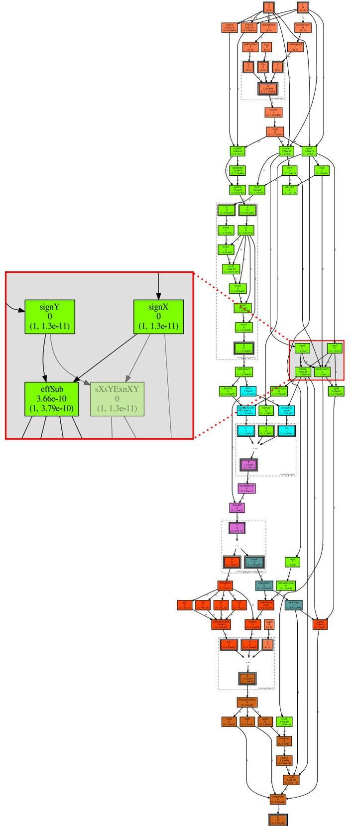
Fig. 5: S-Graph for a single-precision floating-point adder
