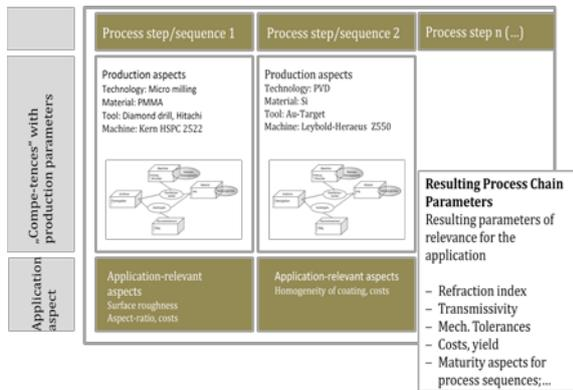
Figure 5: Process sequences in the ProWiDa Methodology
