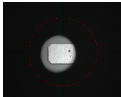
Figure 9: MDA contact pad inside a via hole of the LTCC carrier
