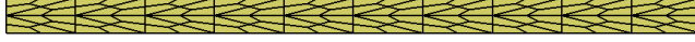
Figure 2: Pseudo one dimensional channel of length L and height H , meshed with strongly distorted elements.
