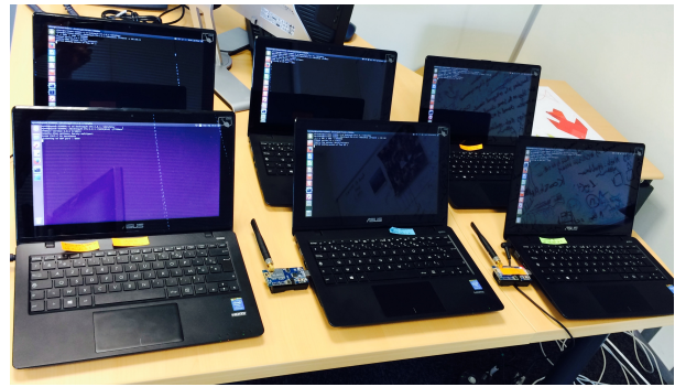
Fig. 5: Experimental setup: 3 pairs of laptops occupy 3 orthogonal channels of Wi-Fi (1, 6, 11)
