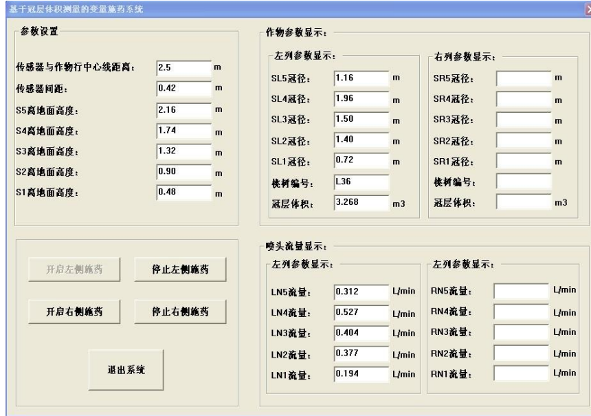
Fig. 10. The working screen capture of variable rate spraying system based on canopy volume measurement.
