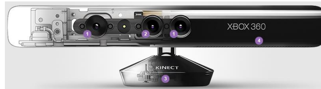
Fig. 1. Composition of the Kinect sensor: (1) - Infrared optics; (2) - RGB camera; (3) - Motorized tilt; (4) - Multi-array microphone
