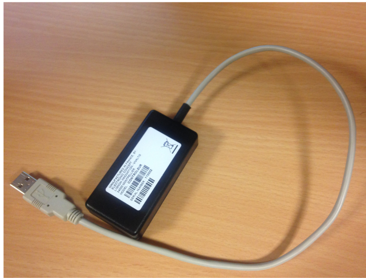
Fig. 3 The communication/control unit of the wireless stimulator
