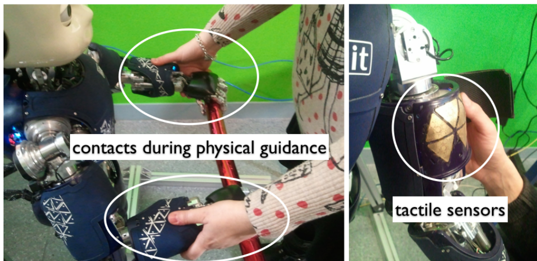
Fig. 4 Demonstration on how to safely grab the robot arms for kinesthetic teaching in the assembly task: the hands of the experimenter grasp the robot forearms on a part covered by the skin. On the left, the distributed tactile sensors underneath the cover.
