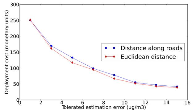
Fig. 1: Optimal coverage cost vs tolerated estimation error.
