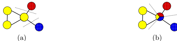
Fig. 1. Partitioning a graph into three clusters, using (a) edge-cut partitioning and (b) vertex-cut partitioning
