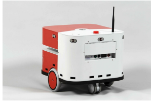
(b) A heavy robot in the smart apartment (Robosoft robuLAB-10, 35.7 kg). Source: www.robosoft.com
