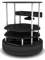
(a) Light robot in the smart apartment (Turtlebot 2, 6.3 kg including notebook). Source: www.turtlebot.com
