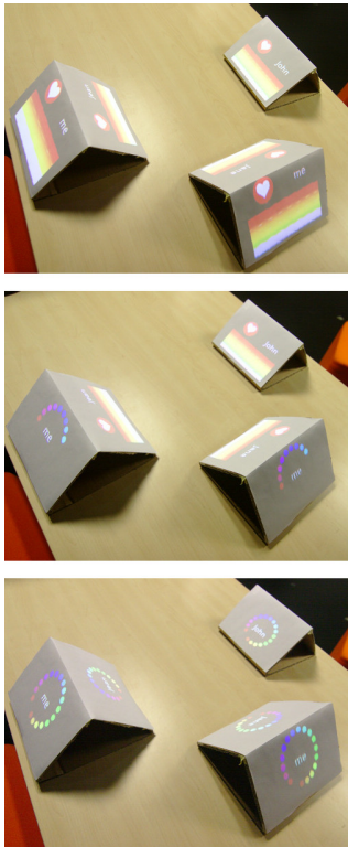
Figure 4: Our experimental conditions regarding heart rate (HR) visualizations. Top: HR visible by all players. Middle: HR visible by the others but not by self. Bottom: HR not visible.
