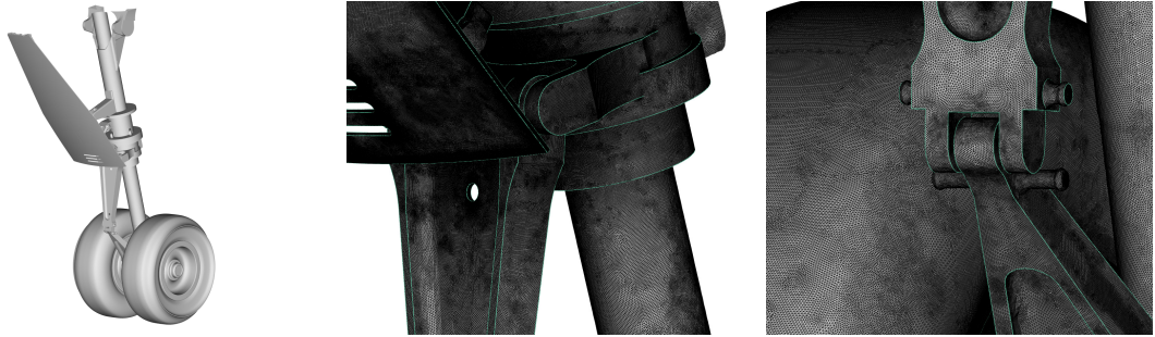
Fig. 8. Landing gear test case. Geometry of the landing gear (left) and closer view of the surface mesh around some geometrical details (middle and right).
