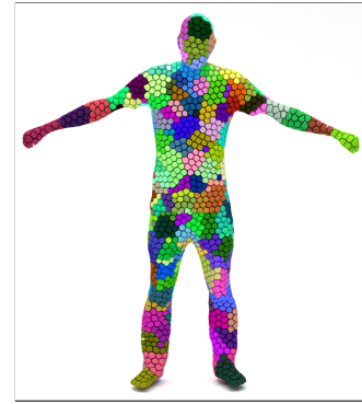
Figure 5: The template model used to recover the runner sequence motion, with its CVT decomposition cells, and the cell clusters in different colors.
