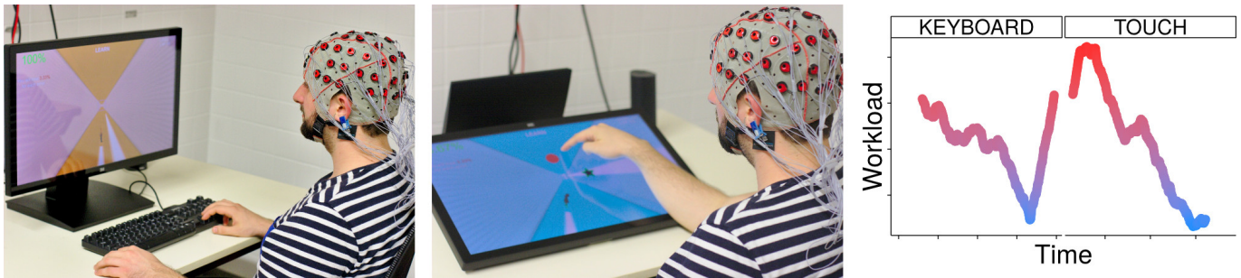
Figure 1: We demonstrate how electroencephalography can be used to evaluate human-computer interaction. For example, a keyboard (left) can be compared with a touch interface (middle) using a continuous measure of mental workload (right, here participant 4).
