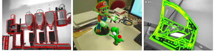
Fig. 8. Markerless model-based tracking [147] [100] [23]: GPU is used to render complex models and to ensure hidden faces removal.
