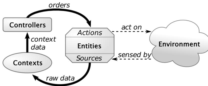
Figure 1: The *Sense/Compute/Control* paradigm, adapted from [9].
