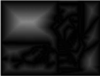
Fig. 7 Distance transform computed from the binary image shown in Fig. 6
