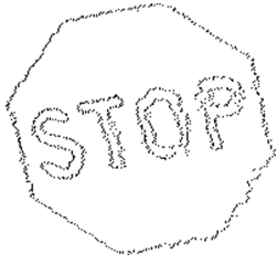
Fig. 10 Rectified 3D contour points computed using Eq. 13 and 14
