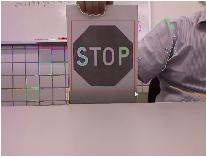
Fig. 12 Template generation application screenshot, where the user selects the object to be detected by drawing a red rectangle around it
