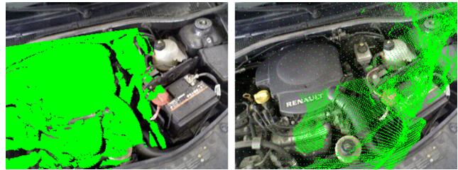
Fig. 26 Non-planar non-smooth object pose estimation is successful when ORB is used (left), while it fails when ORB+DARP is used (right)
