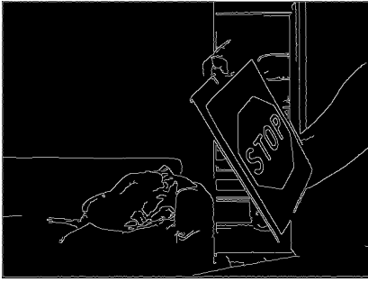
Fig. 6 Canny contour detection example
