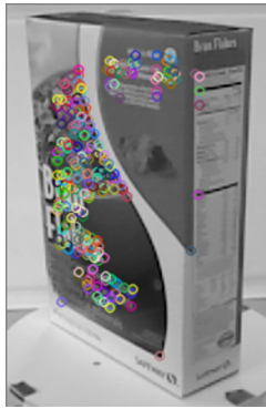
Fig. 2 Keypoint detection example, where each detected keypoint is represented by a colored circle
