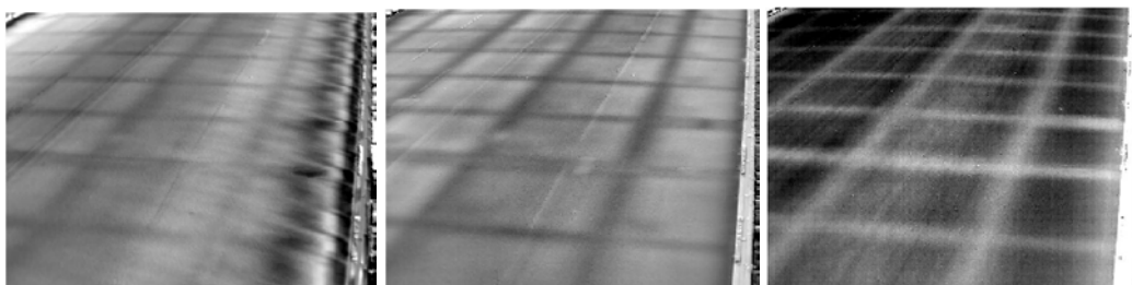
Fig. 5 Full sequence EOF map (left) – Reduced sequence second EOF map (middle) and third EOF map (right).
