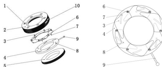
1. hole of hinge axis 2. blade connection seat 3. blade 4. cam ring 5. locked ring 6. hinge axis 7. sliding limited post 8. guiding chute 9. Handle 10. Notch of the connection seat
