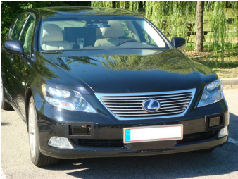
Fig. 6. Experimental platform : Lexus LS600h car equipped with two Ibeo Lux Lidars and cameras.
