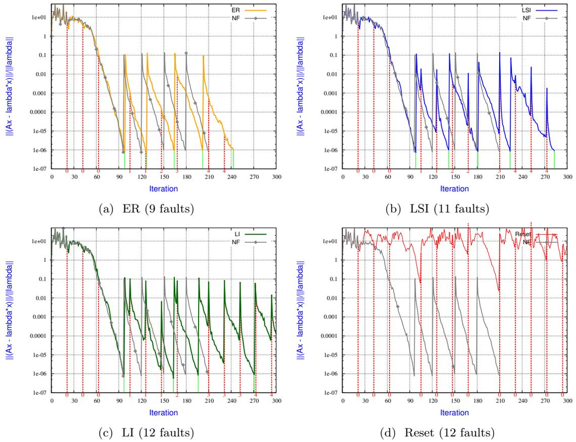
Figure 8: **Comparison of IR strategies** using *nev* regenerated vectors when converging the **five eigenpairs** associated with the **smallest eigenvalues** using **Jacobi-Davidson**. The fault rate is the same for all strategies and a proportion of 0.8 % data is lost at each fault.
