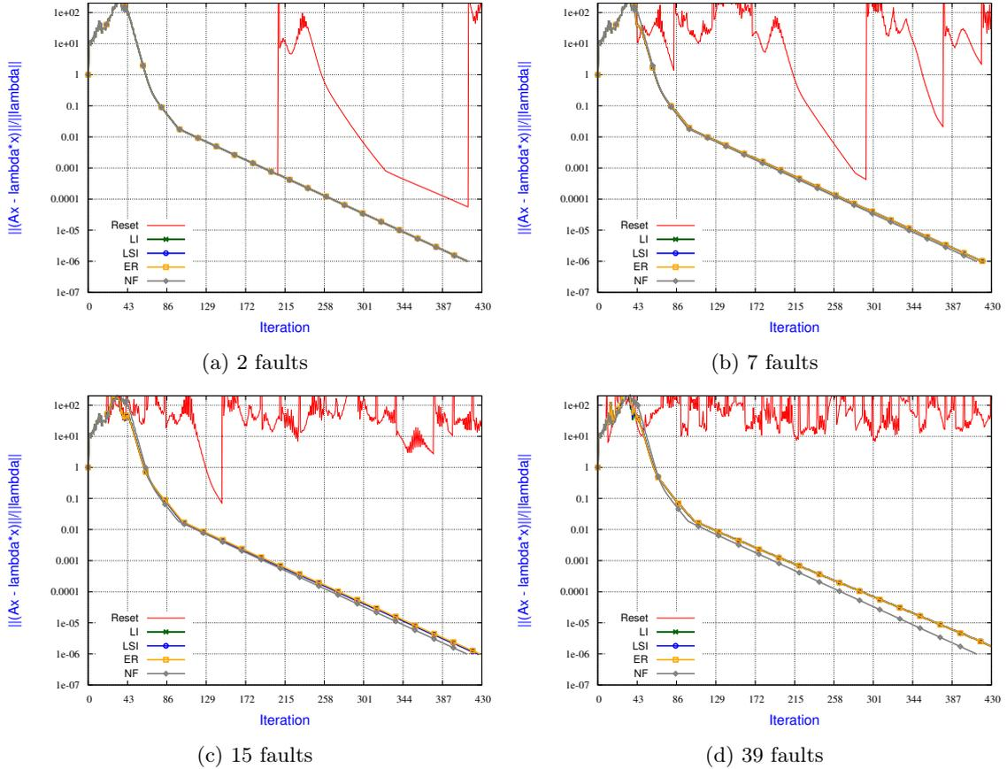
Figure 2: **Impact of the fault rate** on the resilience of IR strategies when converging the **five eigenpairs** associated with the **smallest eigenvalues** using subspace iteration method accelerated with **Chebyshev**. A proportion of 0.8 % of data is lost at each fault. Note that LI, LSI, ER and NF almost coincide.
