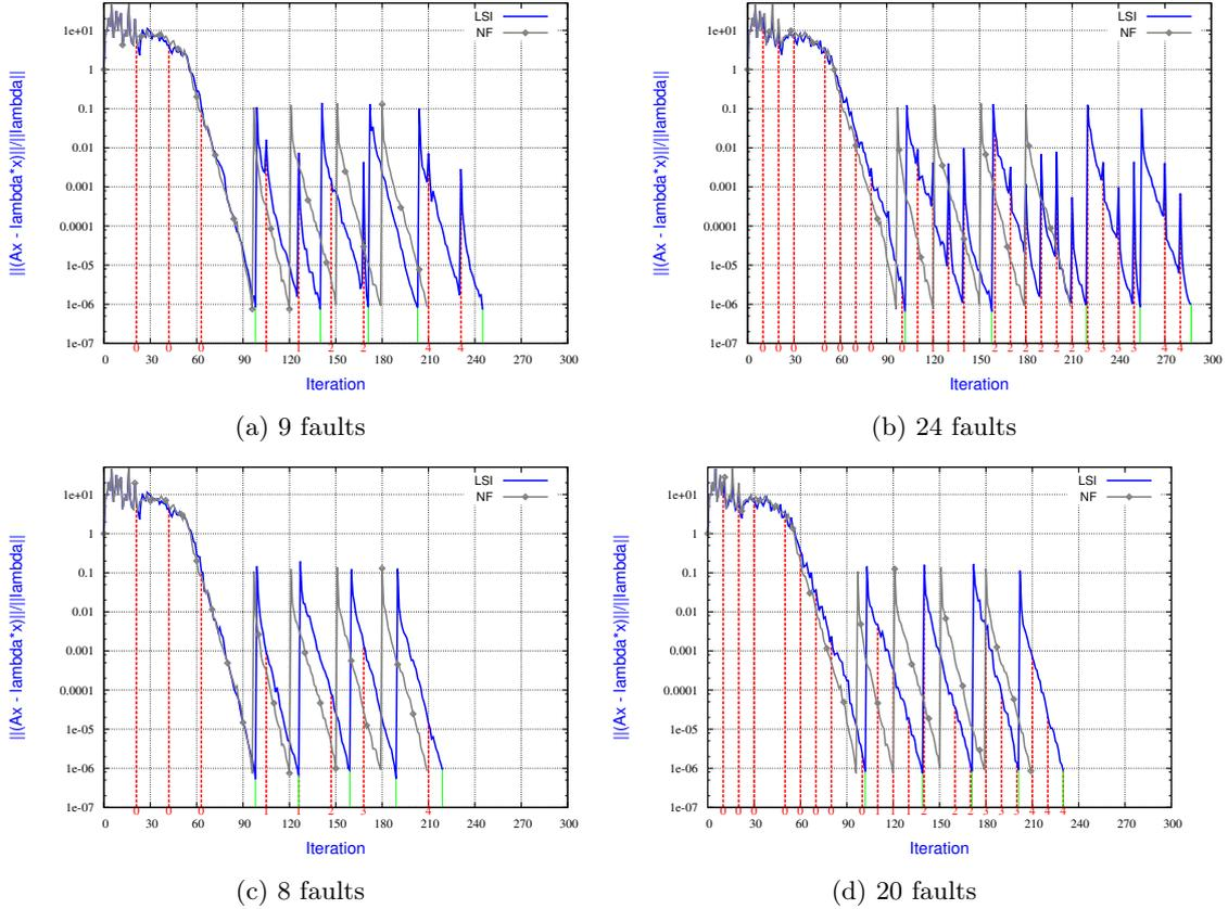
Figure 12: Impact of **keeping the best Schur vector candidate** in the search space after a fault combined with  $nev + nconv - 1$  interpolated directions. Top two plots  $nev + nconv$  interpolated directions, bottom two plots  $nev + nconv - 1$  interpolated directions plus the best Schur candidate. Calculation of the **five eigenpairs** associated with the **smallest eigenvalues** using **Jacobi-Davidson** with a proportion of 0.2 % of data is lost at each fault.
