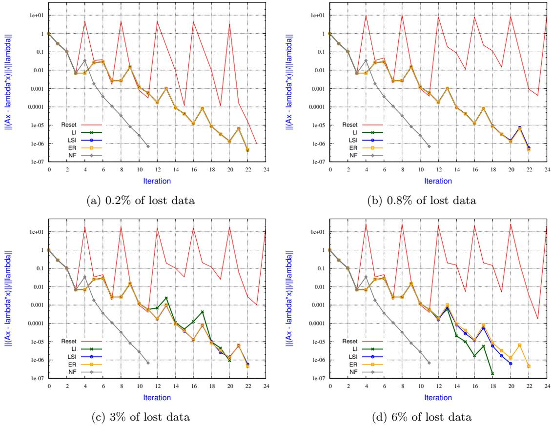
Figure 7: **Impact of the amount of lost data on the resilience of IR strategies when converging the five eigenpairs with largest eigenvalues using IRAM.** The volume of lost data varies from 0.2% to 6% whereas the fault rate is constant. LI, LSI and ER coincide in (a) and (b).
