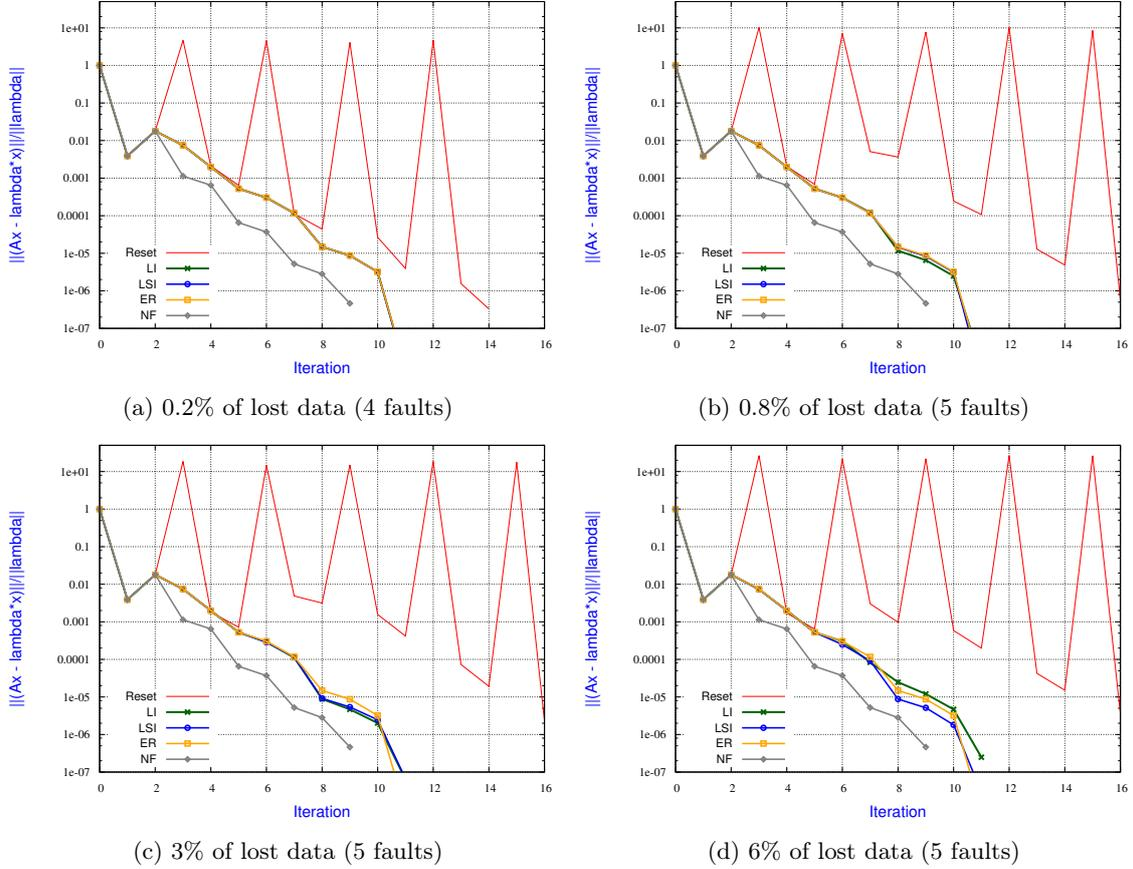
Figure 6: **Impact of the amount of lost data** on the resilience of IR strategies when converging the eigenpair associated with the **largest eigenvalue** using **Arnoldi method**. LI, LSI and NF coincide in (a) (b) and (c).
