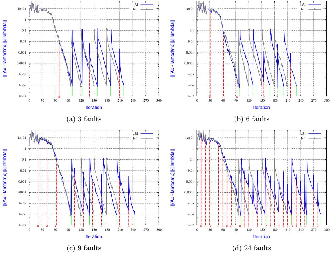
Figure 10: **Impact of the fault rate** on the resilience of **LSI** using  $(nev + nconv)$  regenerated vectors when converging the **five eigenpairs** associated with the **smallest eigenvalues** using **Jacobi-Davidson**. The fault rate varies whereas a proportion of 0.2 % of data is lost at each fault. At each fault, all the already converged Schur vectors are retrieved in the basis of restart.
