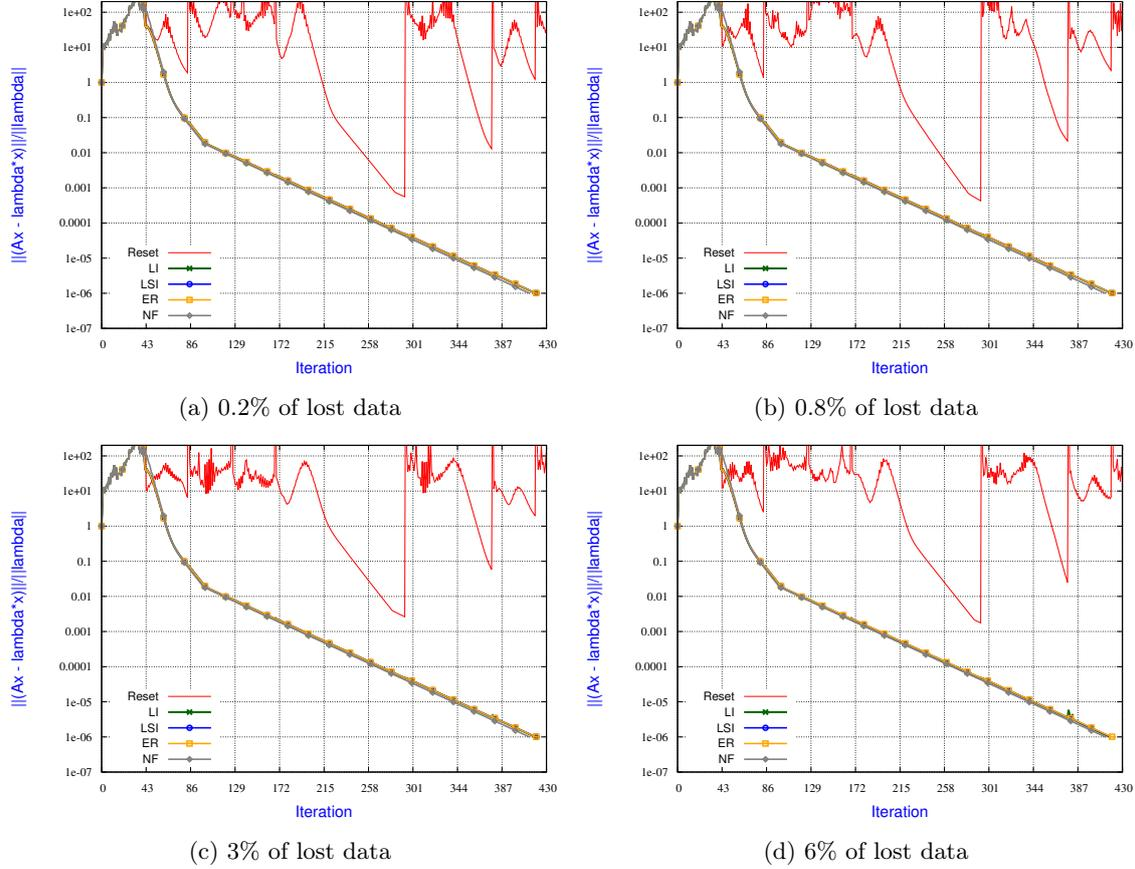
Figure 3: **Impact of the amount of lost data** on the resilience of IR strategies when converging the **five eigenpairs** associated with the **smallest eigenvalues** using subspace iteration method accelerated with **Chebyshev**. The volume of lost data varies from 0.2% to 6% whereas the fault rate is constant (7 faults). LI, LSI, ER and NF coincide.
