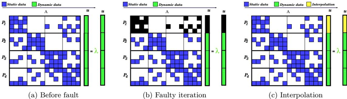
Figure 1: General interpolation scheme. The matrix is initially distributed with a block row partition, here on four nodes (a). When a fault occurs on node  $P_1$ , the corresponding data is lost (b). Whereas static data can be immediately restored, dynamic data that has been lost cannot and we investigate numerical strategies for interpolating it (c).
