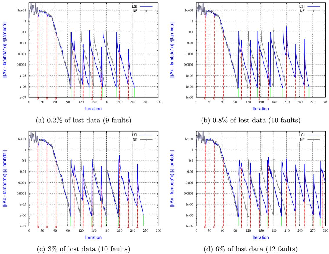
Figure 9: **Impact of the amount of lost data** on the resilience of **LSI** using  $(nev + nconv)$  regenerated vectors when converging the **five eigenpairs** associated with the **smallest eigenvalues** using **Jacobi-Davidson**. The volume of lost data varies from 0.2% to 6% whereas the fault rate is constant. All converged Schur vectors are found immediately after interpolation followed by restart.
