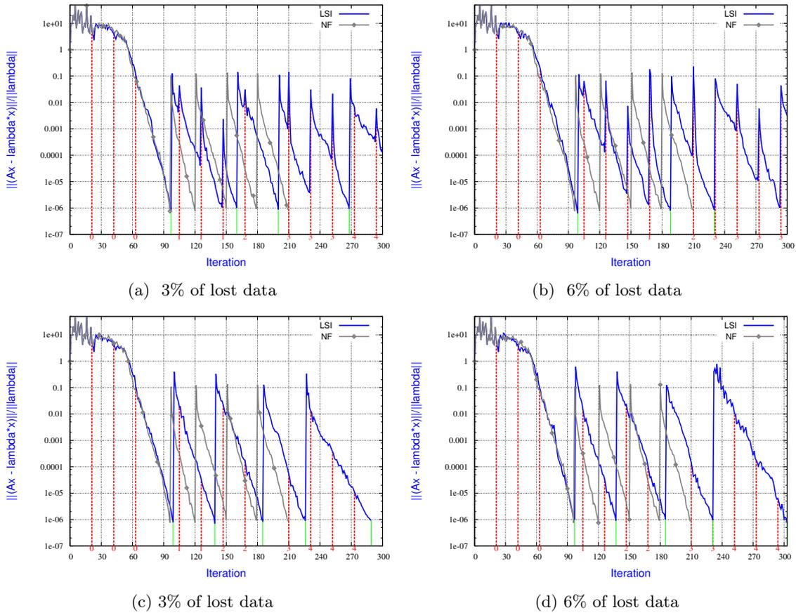
Figure 11: Impact of **keeping the best Schur vector candidate** in the search space after a fault combined with  $nev + nconv - 1$  interpolated directions. Top two plots  $nev$  interpolated directions, bottom two plots  $nev - 1$  interpolated directions plus the best Schur candidate.
